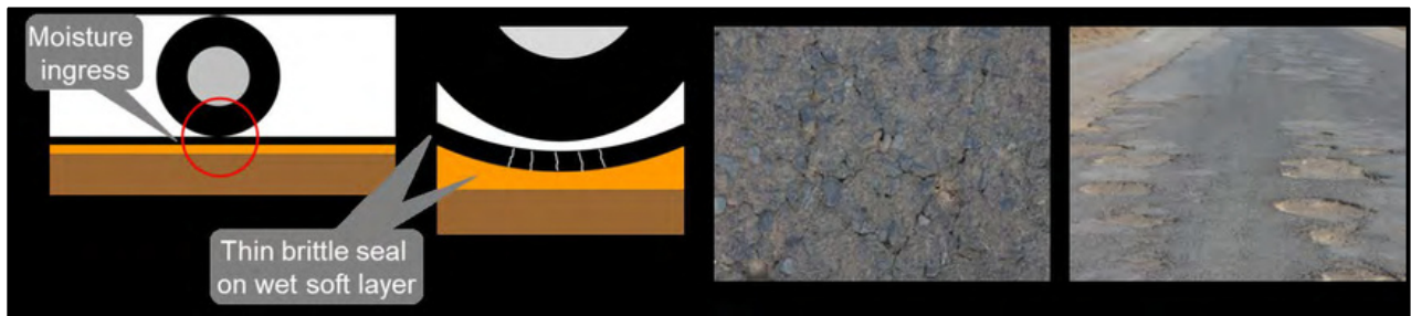
Figure H 6 Moisture ingress resulting in cracking and potholing
